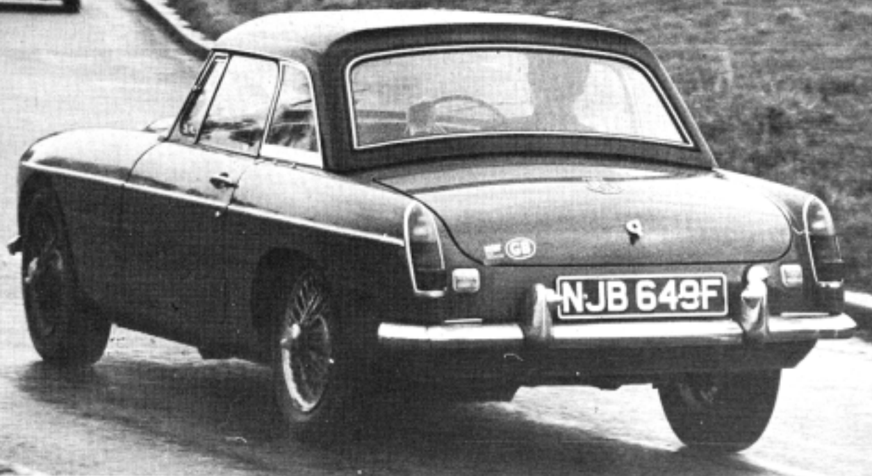
From the rear the MGC is indistinguishable from the MGB, except for a small "MGC" emblem on the boot above the octagon, and wider tyres on 5J rims that not all MGBs have.
