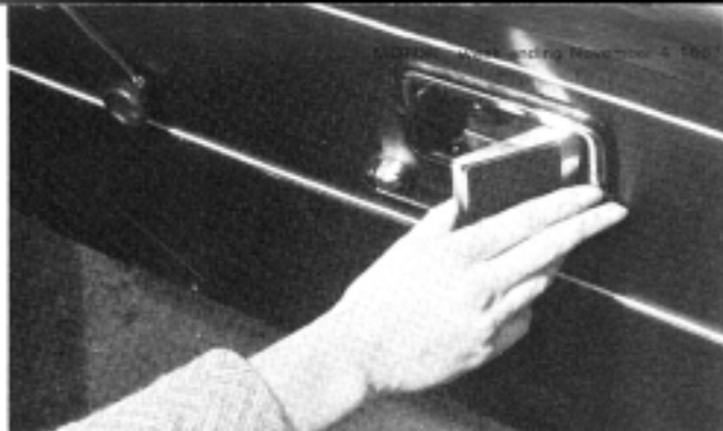
Window winders are made of yielding material, and neatly recessed door locks are a new feature. The plastic tongue at the front of the recess locks the door.
